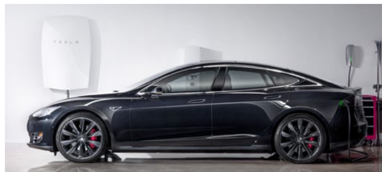
The Tesla PowerWall battery, in the top left of the photo, addresses the problem of the intermittency of wind and solar power. A 7 kWh version is optimised for solar power applications while a 10 kWh version is aimed primarily at backup applications. Round-trip efficiency is claimed to be better than 92%. (Photo courtesy of Tesla)
